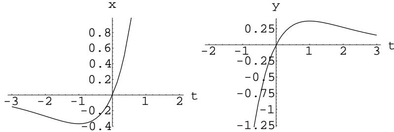
The highest point (maximum  $y$  coordinate) and leftmost point (minimum  $x$  coordinate) seem to occur near  $t = 1$  and  $t = -1$ , respectively. A quick calculation shows that indeed  $dy/dt = (1-t)e^{-t} = 0$  if  $t = 1$ , and  $dx/dt = (1+t)e^{-t} = 0$  if  $t = -1$ . The parametric curve, in a slightly exaggerated graph, looks as follows:
