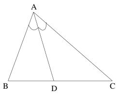
The Internal Angle Bisector Theorem states that if AD is an internal angle bisector of  $\angle BAC$ , then  $\frac{AB}{AC} = \frac{BD}{DC}$ .
