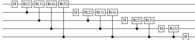
The input qubits of the circuit above use a big-endian ordering. We can convert to little-endian ordering by reversing the input vector.
