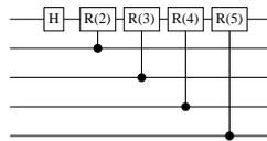
To construct such a circuit in Proto-Quipper-D, we first define the `rotate` function, which will produce a cascade of rotations with a single target. The rotations in the above circuit are then generated by `oneRotation 4`.
